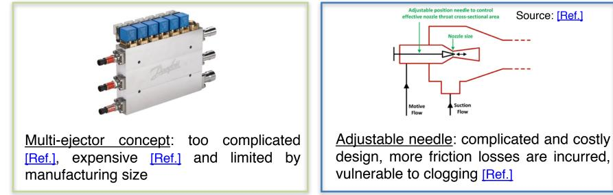
At present, two-phase ejectors cannot be effectively capacity controlled without penalizing ejector and system efficiency in small-scale HVAC&R units
