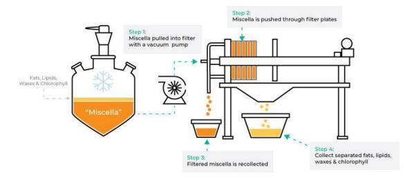
**Figure 16.** Cannabis Filter Press device for post-winterization filtration of miscella or crude cannabis oil, as well as fines filtration. The press has the option to add up to 5 more filtration plates, easily doubling the throughput. This is great for scalability, making it a reliable fit for labs of all sizes and production capacities in need of cannabis filtration.
