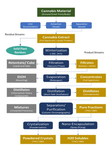
**Figure 15.** Schematic diagram of Supercritical fluid extraction with CO<sub>2</sub> and downstream processing steps for producing purified cannabis-based products.
