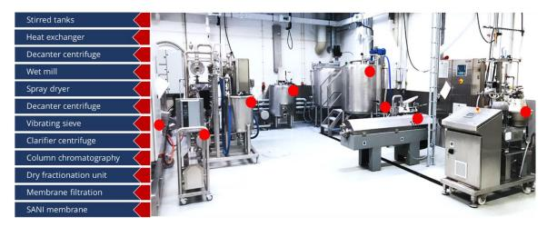
**Figure 1.** Generic cascading unit operations for upcycling plant biomass utilized in the ProEnrich project.
