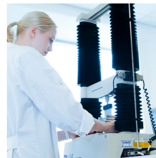
Warner Bratzler shear force. All samples were aged for 72 hours at 5°C before freezing.
