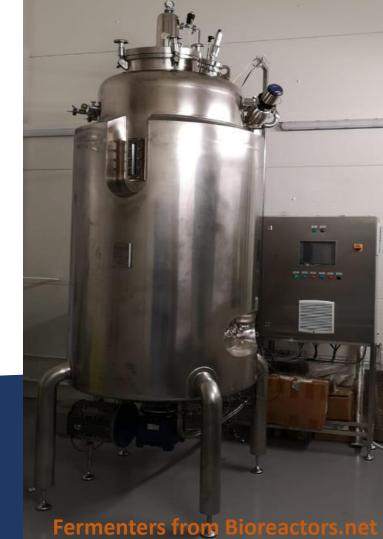
**Gas supply** controlled by MFC; ring sparger; gas mixing chamber.
