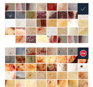
AI SURFACE CHECKER detects contaminations on the varying carcass background.
