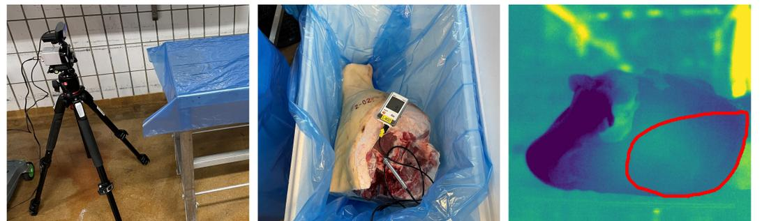
Figure 1a. Camera setup used to obtain thermographic images (A), placement in flamingo boxes for adiabatic equalisation (B) and manually annotated pixel region corresponding to *M. gluteus profundus*, *M. gluteus medius* and *M. gluteus accessorius* used to calculate  $T_{surf}$  (C).
