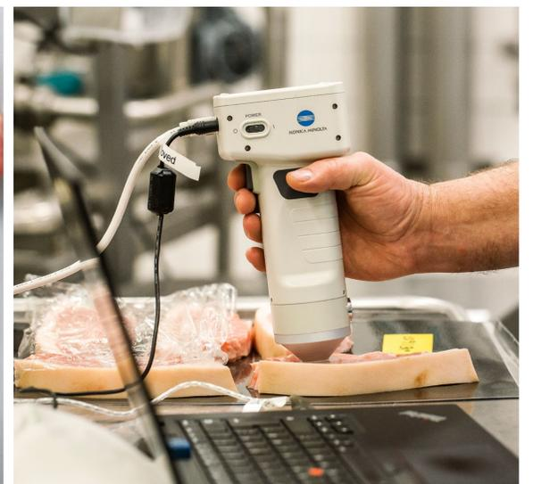
Figure 1e. Measuring Minolta colour.
