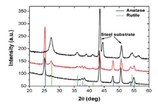
Figure 3: X-ray diffractograms from 1 µm TiO2 coatings deposited on stainless steel substrate. The diffractograms reveal coatings consisting of the crystal phases anatase (bottom), anatase + rutile mixture (middle) and rutile (top), respectively.
