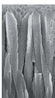
Figure 2: Cross section of an anatase TiO<sub>2</sub> coating seen with a scanning electron microscope. The coating thickness is about 1 µm.
