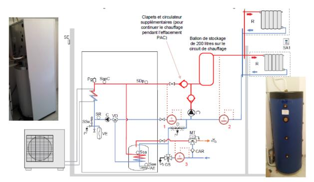
Figure 57: HP installation in Losange Project
