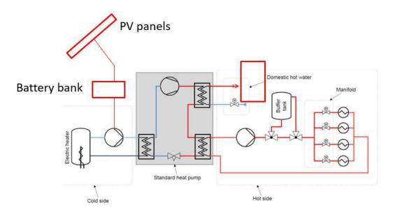
Figure 65: Sketch of experimental setup (on the test rig PV and battery are virtual).
