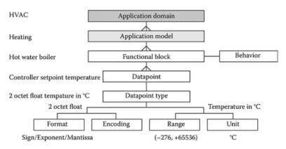
Figure 18: Example of KNX application modeling. Source: (Ruta, Scioscia, Loseto, & Di Sciascio, 2015).
