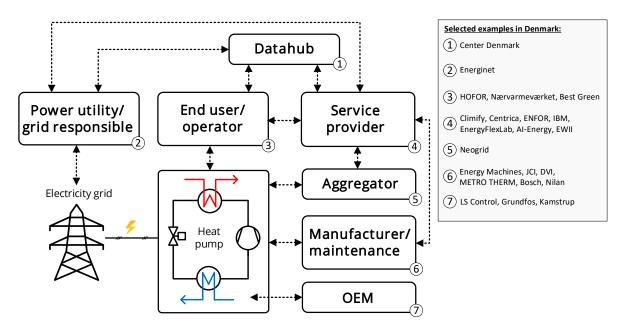
Figure 84: Visualization of supplier groups and examples of associated suppliers in an IoT-based energy system for heat pumps.
