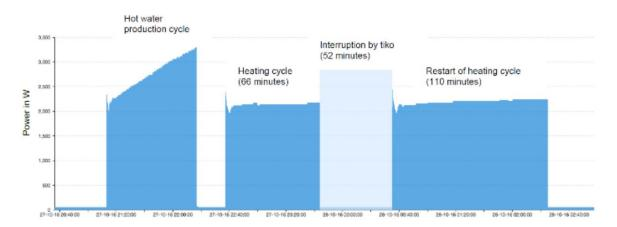
Figure 55: Heat pump cycle interrupted by tiko control
