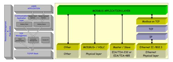
Figure 16: MODBUS Messaging Service Conceptual Architecture and communication stack. Source: (Belliardi & Neubert, 2015).
