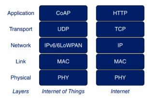
Figure 20: CoAP protocol stack vs. HTTP protocol stack.
