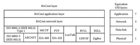
Figure 19: BACnet data-link layers in the ISO/OSI model. Source: (Schubert, 2015).
