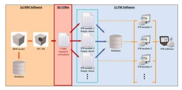
Figure 34: Transfer of building data between BIM and FM software by COBie Standard (Tu and Chang 2017).
