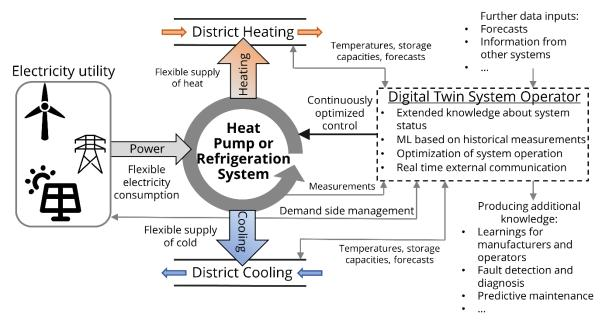
Figure 61: Diagram of the digital twin system operator.
