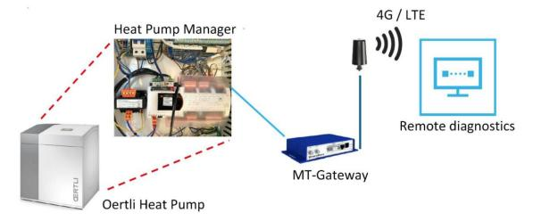
Figure 56: SmartGuard system setup
