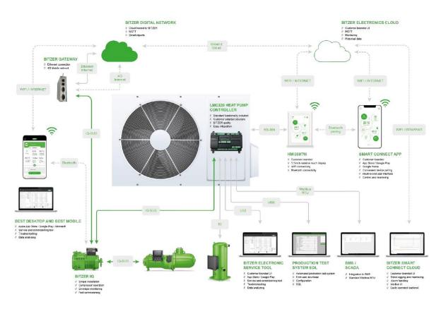
Figure 39: Overview of the Bitzer Heat Pump Ecosystem
