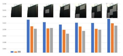
Figure 48: Acceleration measurements visualized as vertical bar charts for artificial ice coverage as shown in the images. The first set show the level of vibration with the fan not operational.
