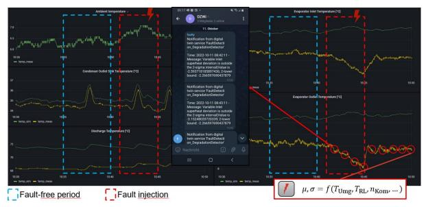
Figure 59: First results of fault detection service for evaporator fouling and resulting user notification.
