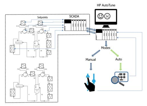
Figure 67: Diagram of the HP AutoTune concept.
