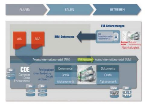
Figure 32: FM-Requirements in a BIM process (GEFMA 2017).
