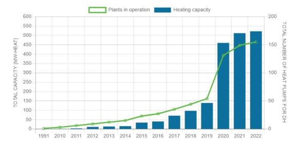
Figure 85: Overview of large-scale heat pumps for the Danish district heating network (Danish District Heating Association, 2022a).
