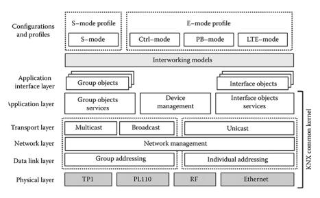
Figure 17: KNX protocol stack and reference architecture. Source: (Ruta, Scioscia, Loseto, & Di Sciascio, 2015).
