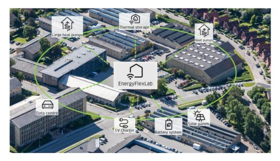
Figure 82: Main energy components in EnergyFlexLab.
