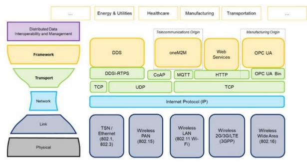
Figure 21: IIoT connectivity stack. Source: (IIC and I4.0, 2017)
