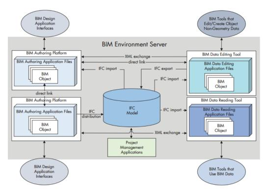
Figure 31: Example of IFC role in a BIM environment. Source: (Sacks, Eastman, Lee, & Teicholz, 2018).
