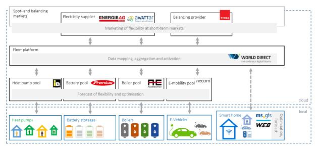
Figure 46: Overview on Flex+, interaction and data processes between stakeholders
