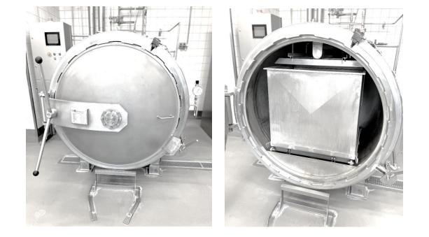
Volume of container: 63×81×95 cm Irrigation autoclave Cooling with cooling water Temperature range: 5 – 140°C Pressure: up to 6 bar Data logging of time, temperature and pressure
