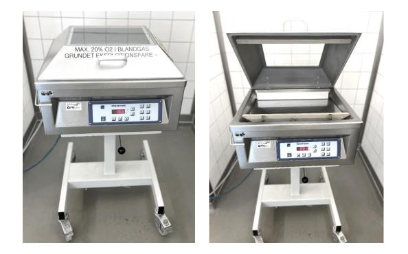
Vacuum packaging - vacuuming degree can be regulated.
